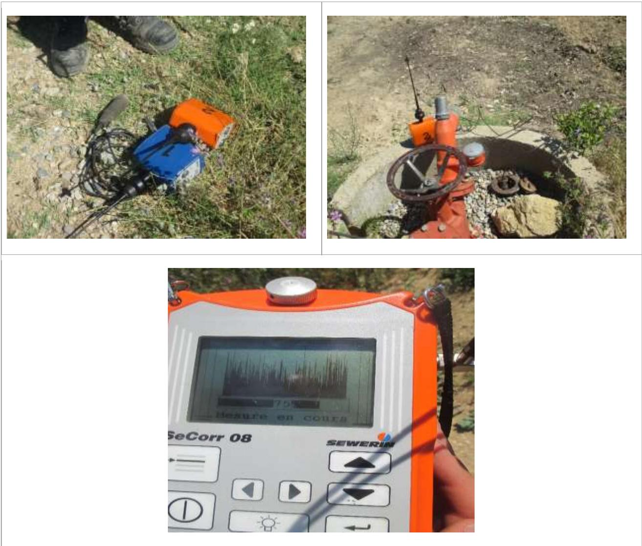
Figure 50 : devices for acoustic correlation method
