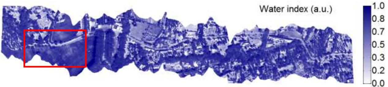
Figure 94 : Water Index (WI) map as obtained from the scaling of brightness temperature defined by the cold and wet edges in the previous figure. Next figure corresponds to a close-up of the area with the leak.
