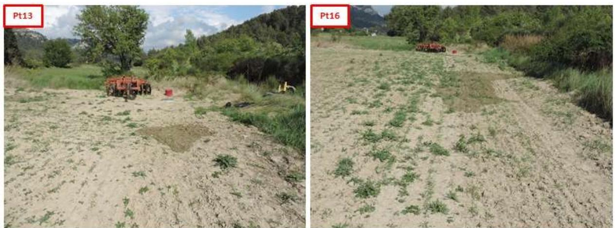
Figure 45: Vauvenargues area: pictures of the soil on the site of controlled leakages (flow rate: 720 l/h).
