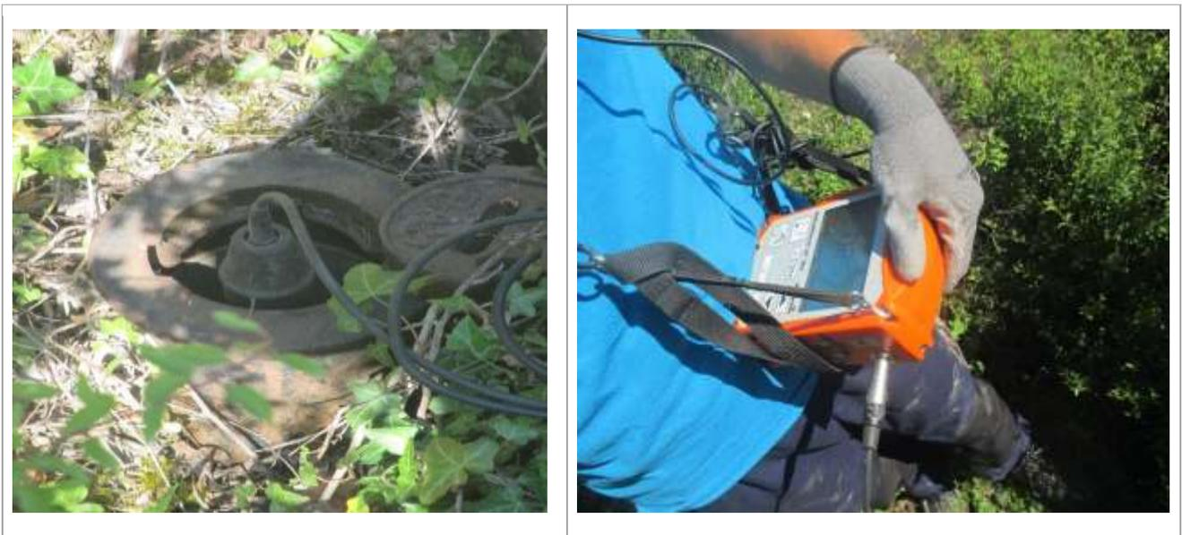
Figure 47 : microphone used for leak detection
