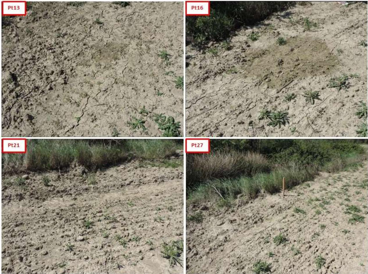
Figure 44: Vauvenargues area: pictures of the soil on the site of controlled leakages (flow rate: 300 l/h).
