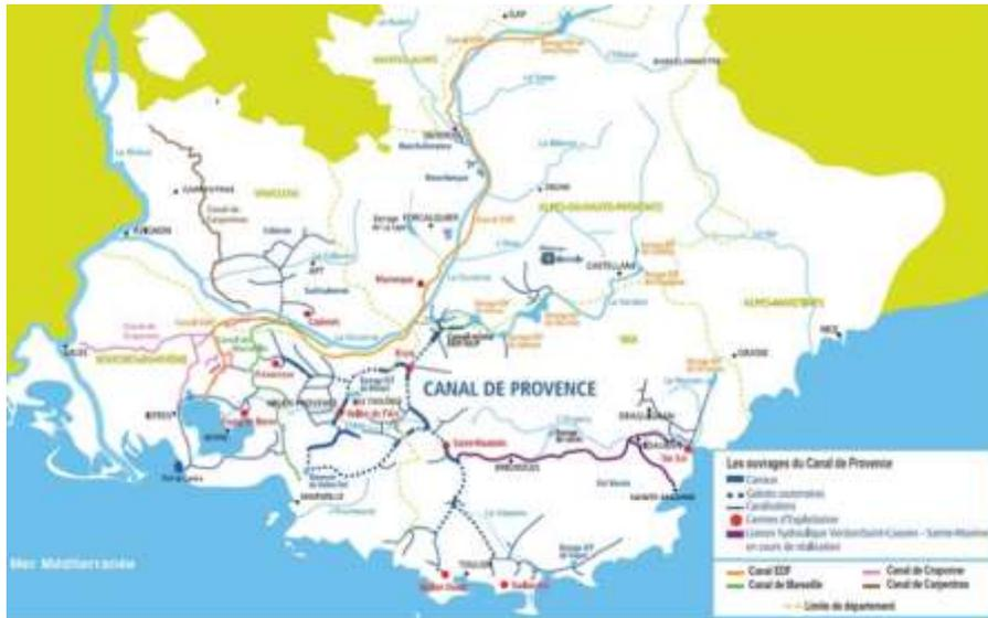
Figure 23: Water network infrastructure provided by SCP
