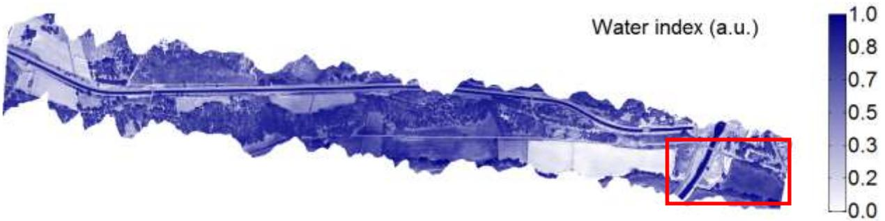
Figure 103 : Water Index (WI) map as obtained from the scaling of brightness temperature defined by the cold and wet edges in the previous figure. Next figure corresponds to a close-up of the area with the leak.
