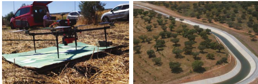
Figure 3 : Airborne & UAV platform equipped with WADI sensors system
