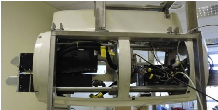
Figure 2-3 Hypspx VNIR and SWIR hyperspectral cameras integrated in the left pod
