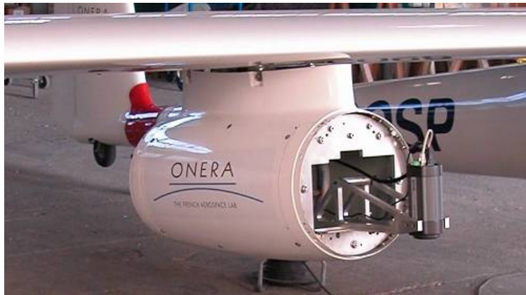
Figure 2-2 FLIR A325 IRT camera mounted in the right pod
