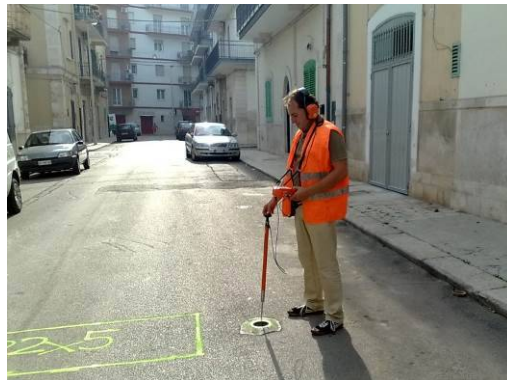
Figure 1-6 Engineer using an electroacoustic listening rod for Direct Sounding
