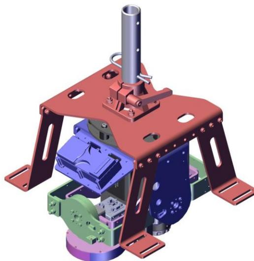
Figure 3-3 New designed geo-stabilized platform
