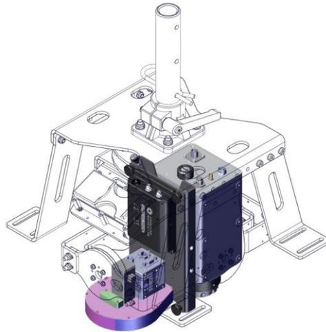
Figure 3-12 Sensor Column with cams and IMU
