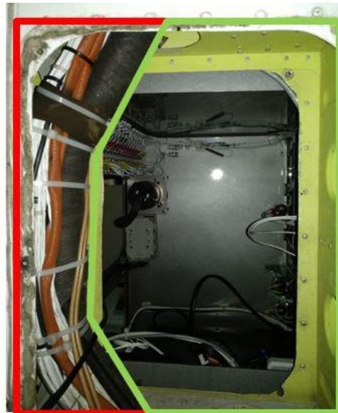
Figure 3-14 Window dimensions after taking into account the cables problem. It's rather a trapezoid.
