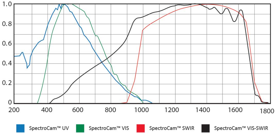
Figure 2-3 Pixelteq SpectroCam spectral response
