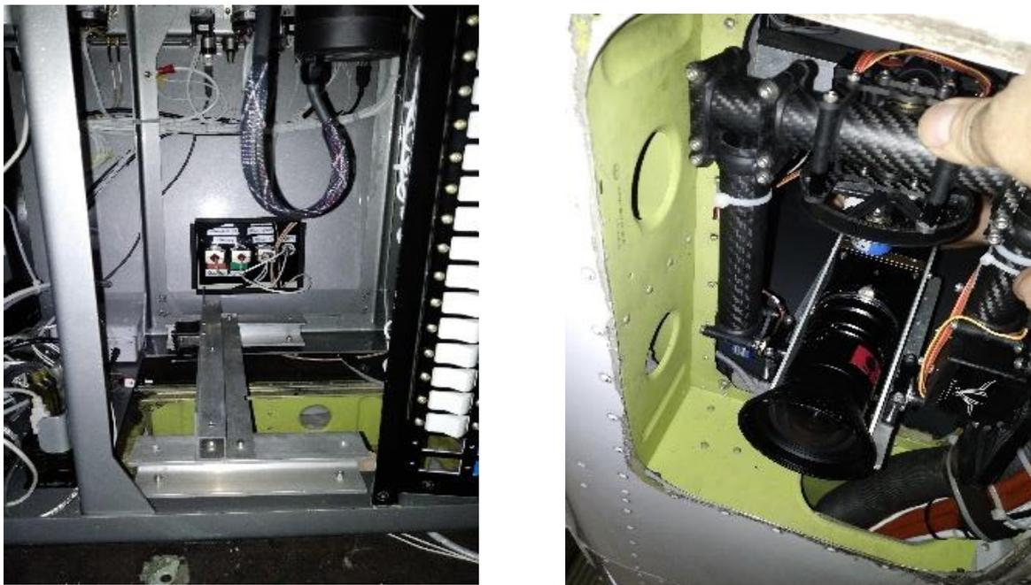
Figure 3-1 Upper access to fuselage hatchway and bottom view gyro-mount embedment.
