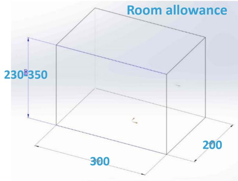
Figure 3-2 Window dimensions for installing the gimbal.
