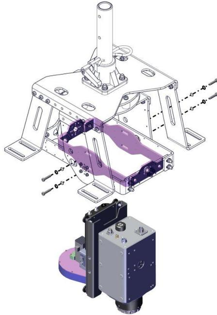
Figure 3-11 Disassembly of sensor column
