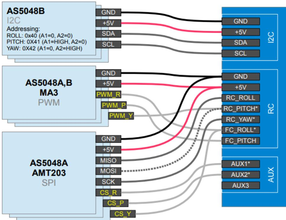
Figure 2-11 BaseCam BGC Pro. Board encoders connection.
