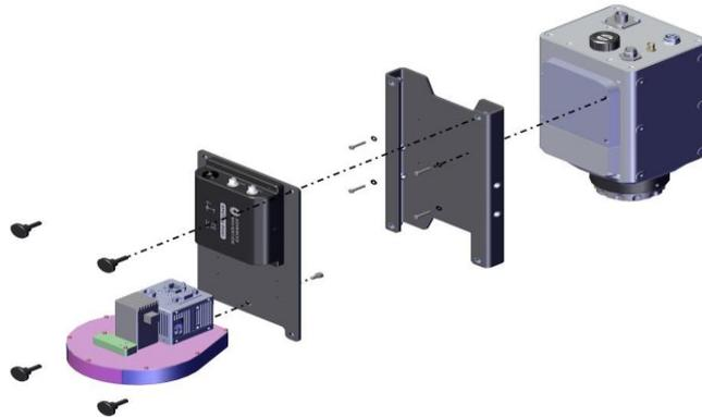
Figure 3-13 Disassembly cams and IMU
