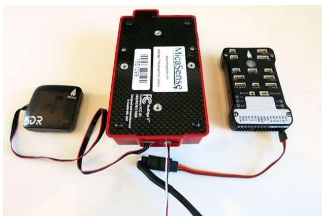
Figure 4. 10 GNSS, MC and autopilot integration and pin connections details
