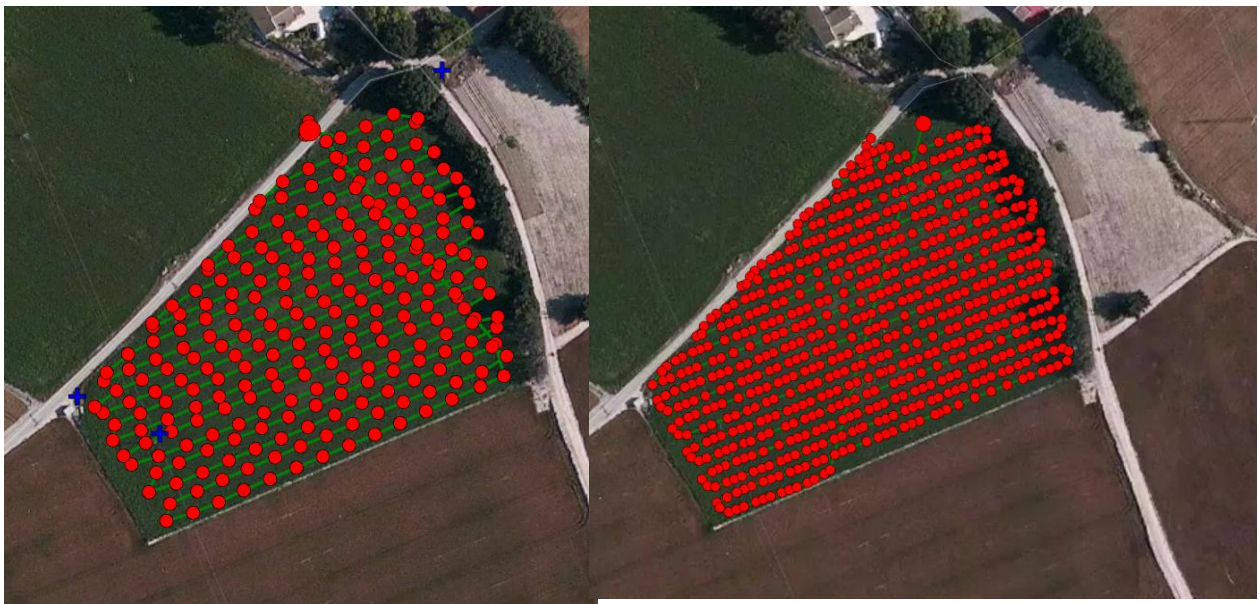
Figure 18. Multispectral (left) and TIR (right) flight paths with camera triggers.
