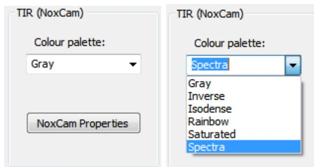
Figure 4 - Colour palette configuration for the NoxCam thermal IR camera
