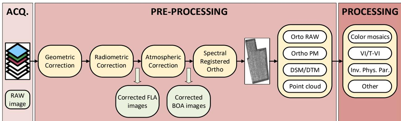
Figure 1 - Data processing pipeline.
