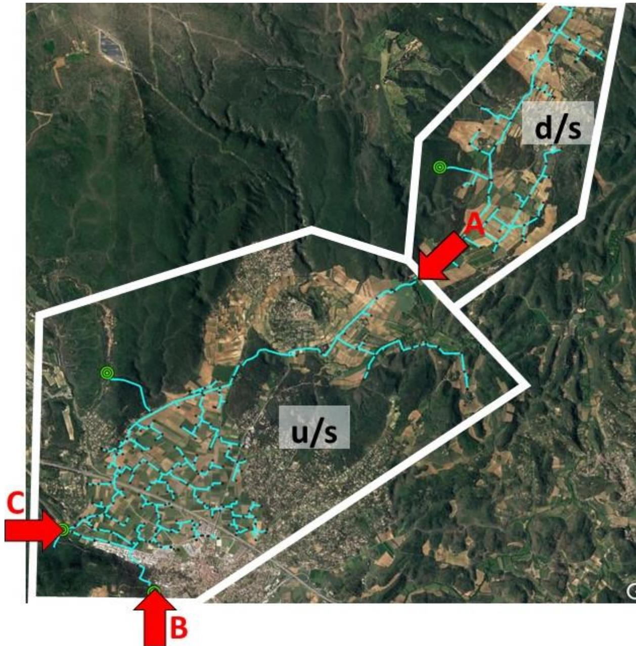
Figure 4.7 Location of the valves to be closed for isolating the two sub-sites.
