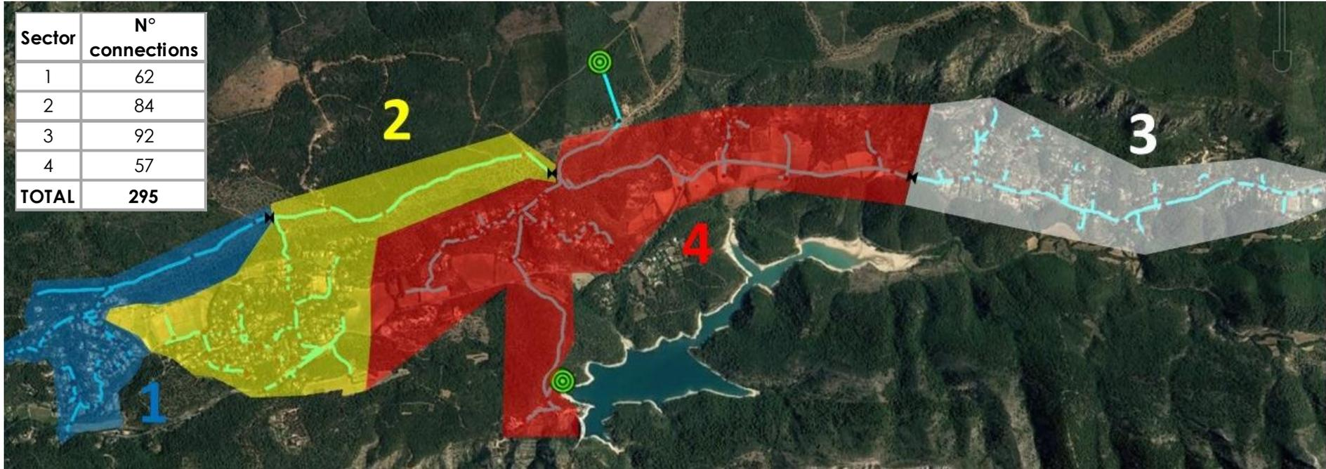
Figure 4.5 Step test plan for Vauvernagues site.
