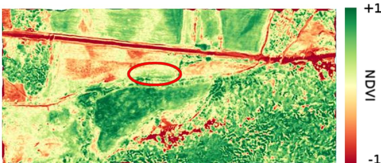
Figure 8.1 NDVI orthomosaic from the waterleaks test field (October 2018).
