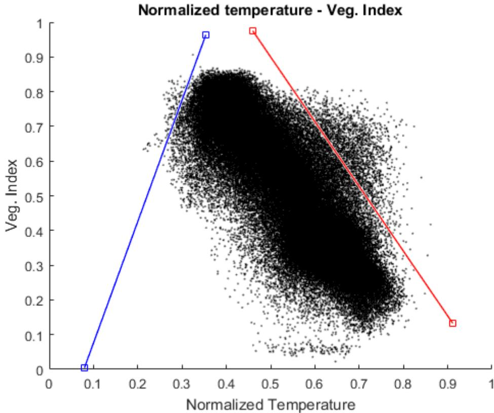
Figure 8.8 - Scatter diagram between the normalized temperature and the NDVI (840 – 668 nm) vegetation index (July 2018).
