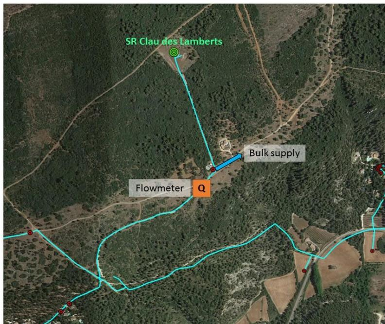
Figure 4.3 Flowmeter installation at Clau des Lamberts SR as per option 1.
