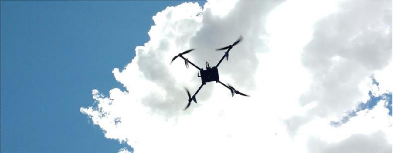
Figure 3.2 Multicopter with on-board multispectral and thermal infrared cameras operated by Galileo Geosystems.
