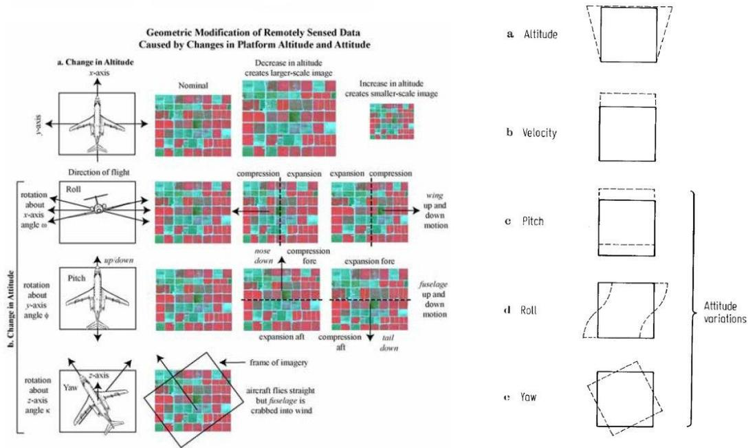
Figure 2.5 Geometric distortions of imagery from airborne sensors.
