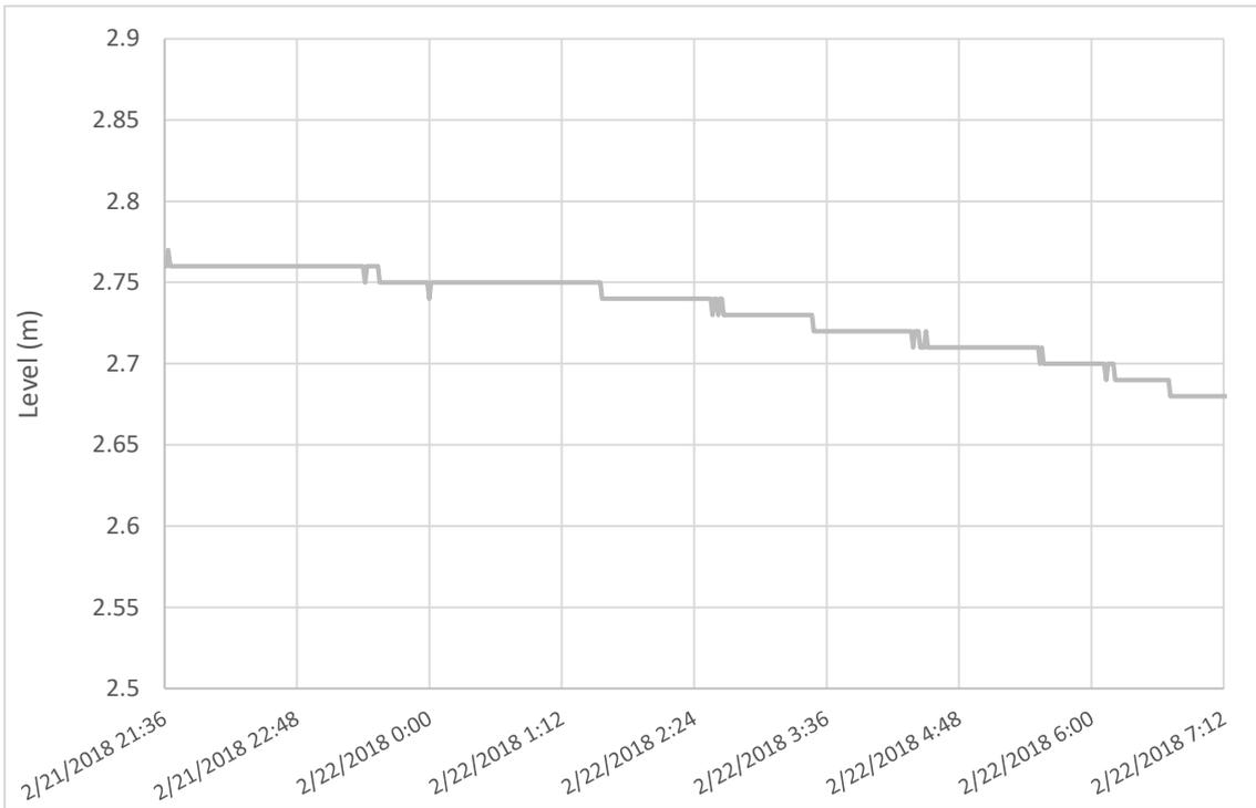
Figure 6.14 Levels measured in Rabinets reservoir during the first night.
