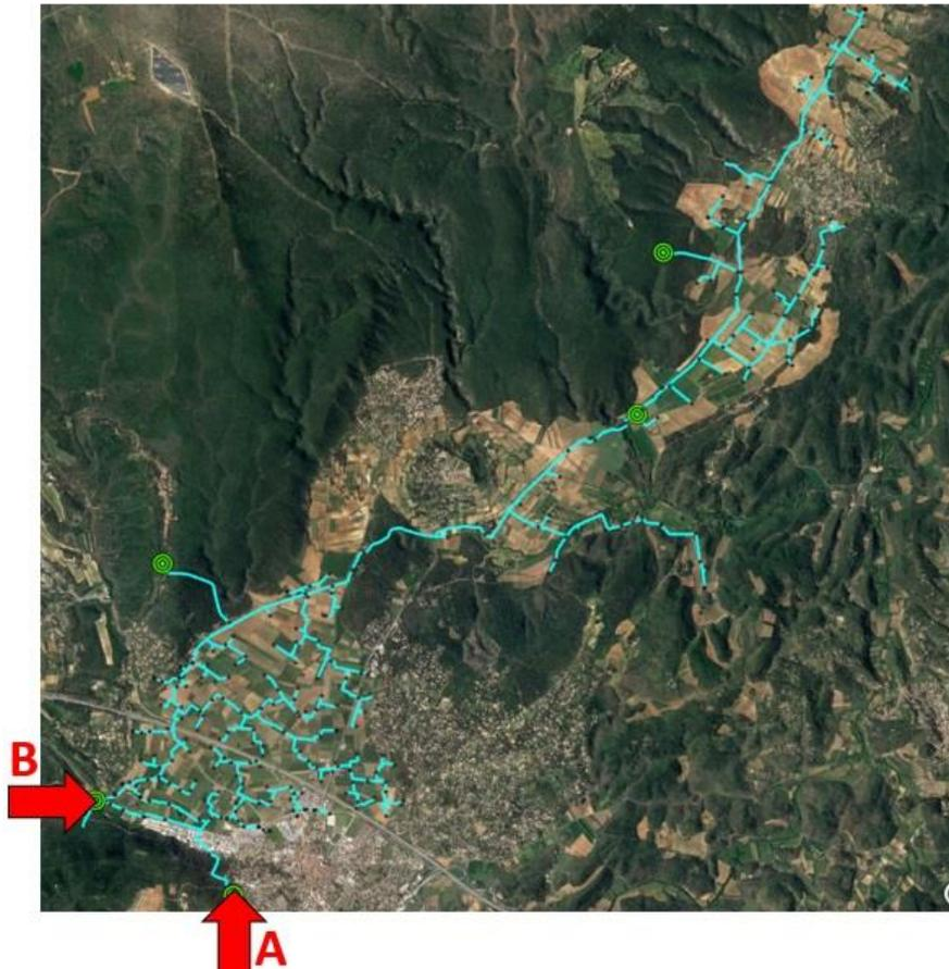
Figure 6.8 Location of the valves closed for isolating the site.
