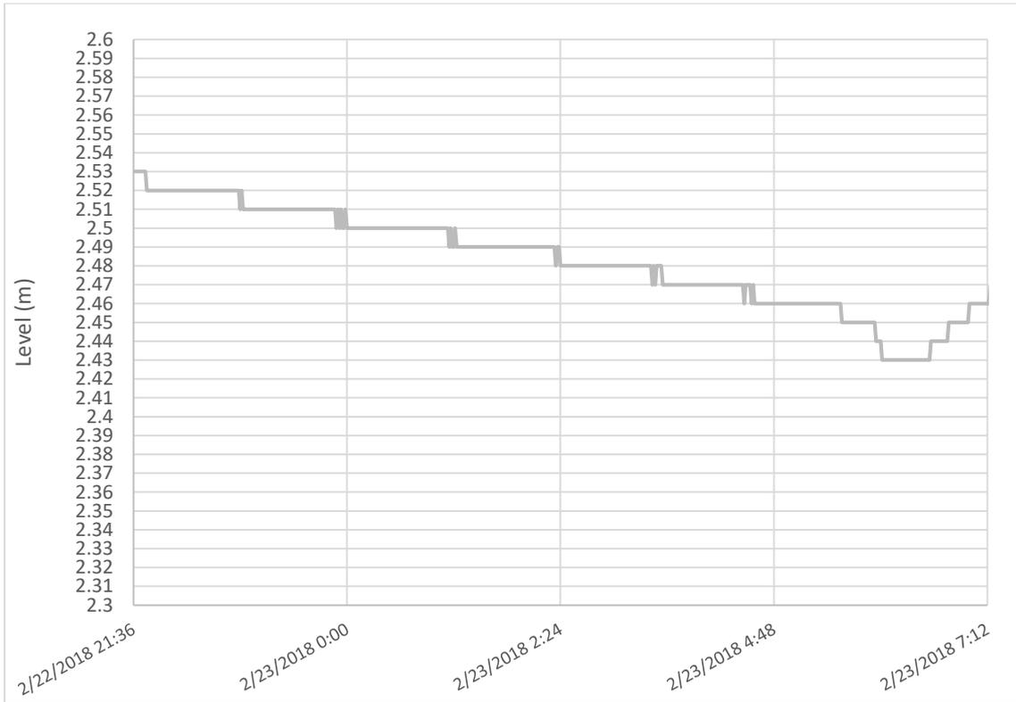
Figure 6.18 Levels measured in Rabinets reservoir during the second night.
