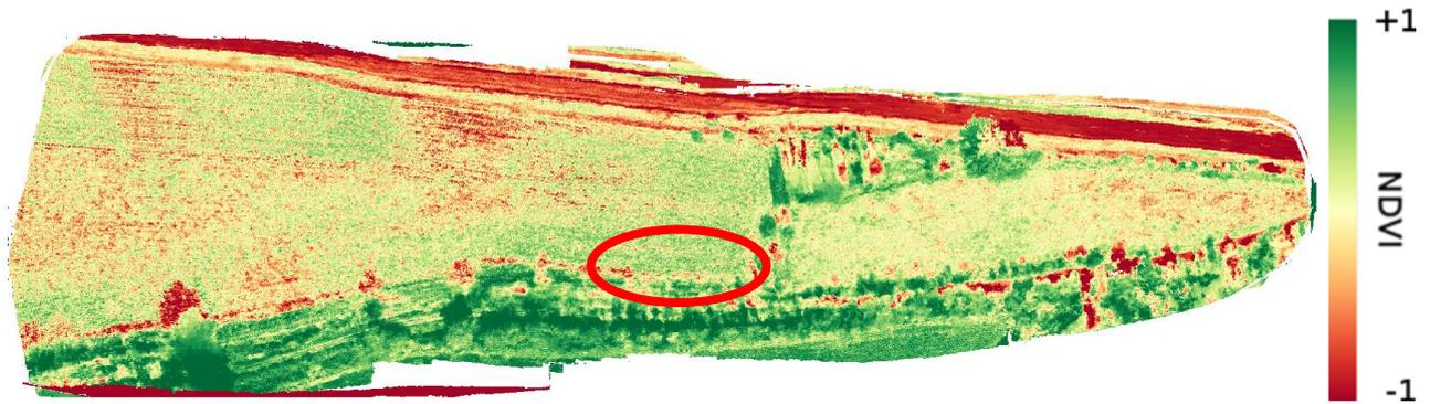
Figure 8.4 NDVI orthomosaic from the waterleaks test field acquired with RPAS (October 2018).
