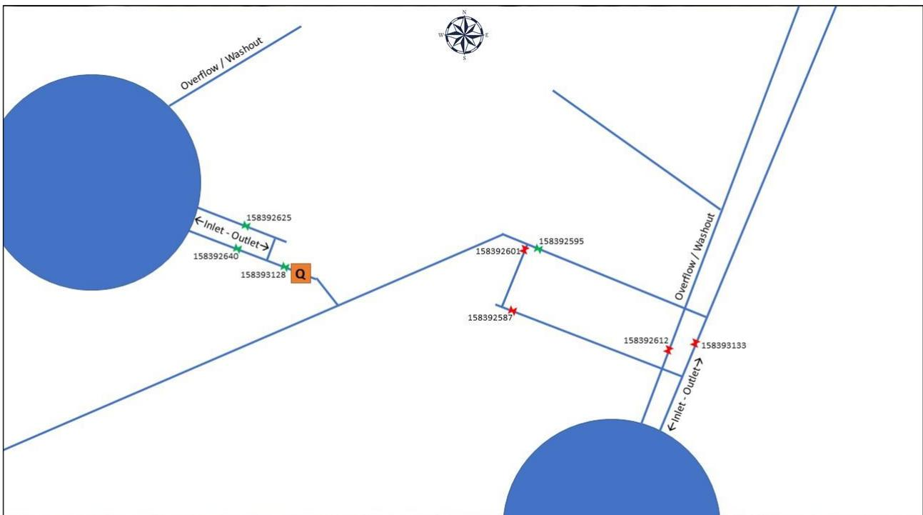
Figure 4.1 Initial valves' configuration (red = closed, green = open) and flowmeter installation point at Cazeneuve SRs.
