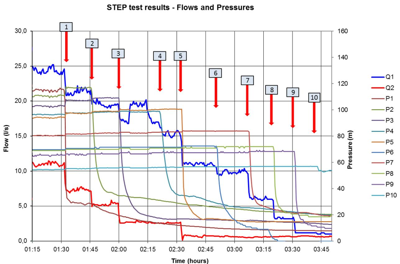
Figure 2.2 Expected results of a step test carried out with the isolation method.
