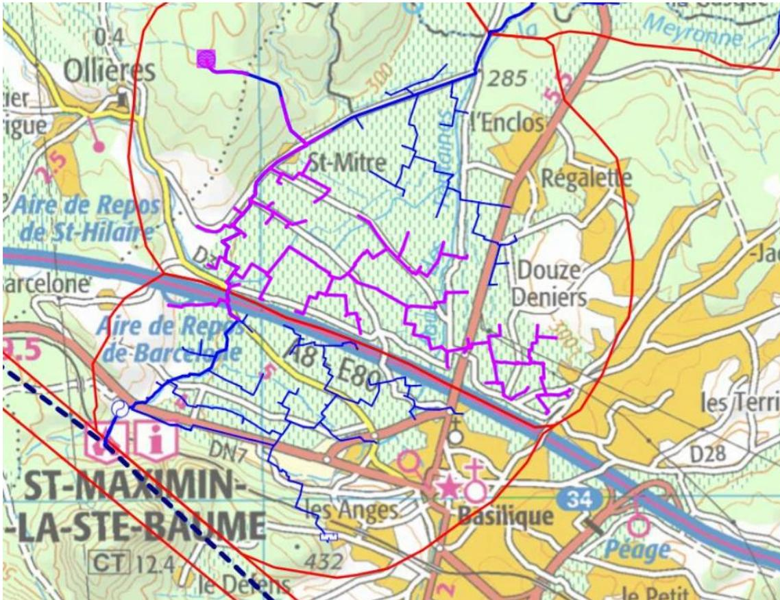
Figure 6.15 Sector 3\* showing the highest leakage rate during the first night.
