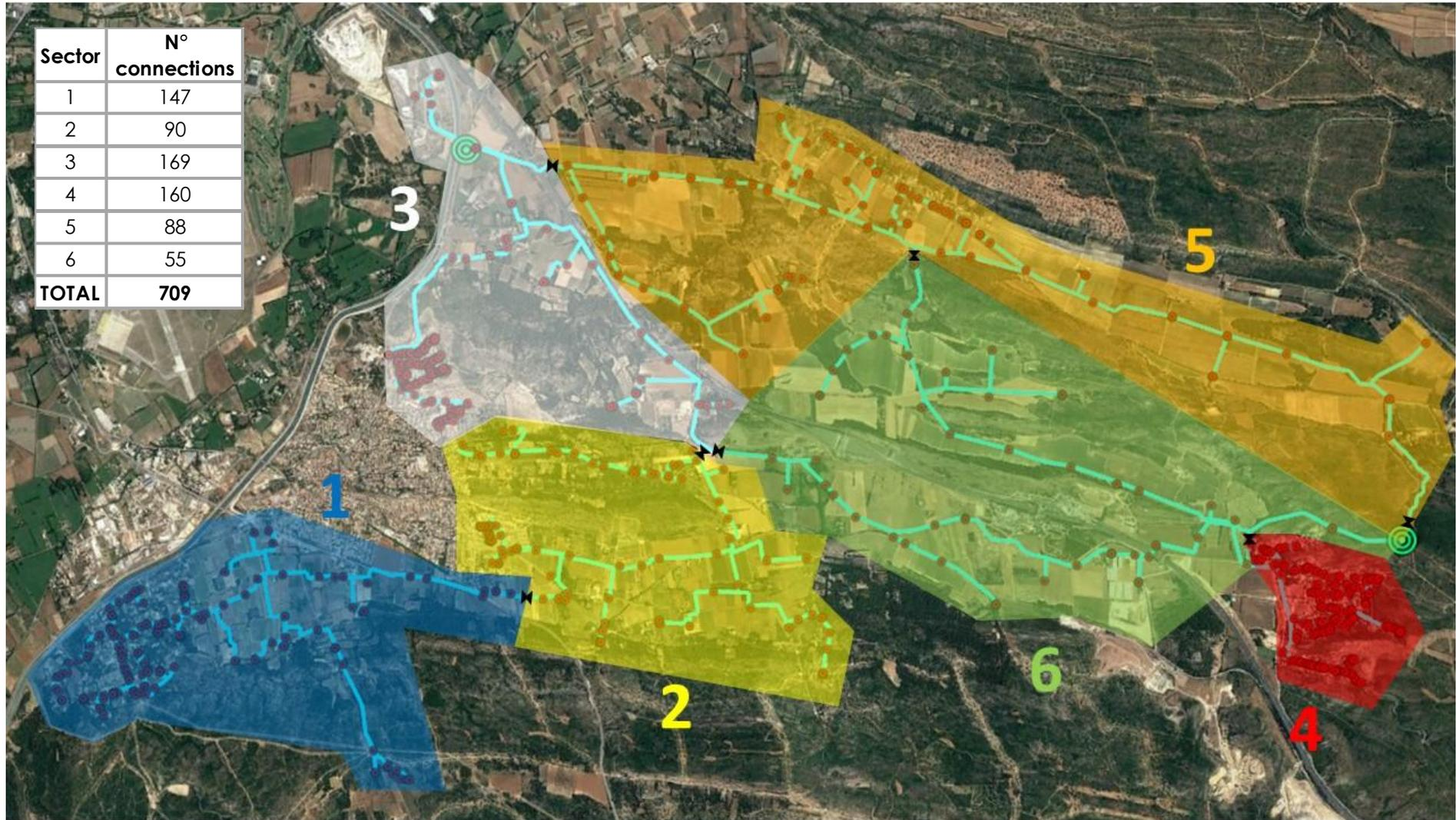
Figure 4.2 Step test plan for Cabardèle site.
