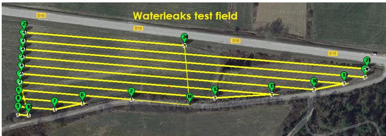
Figure 3.9 RPAS flight plan for the waterleaks test field.
