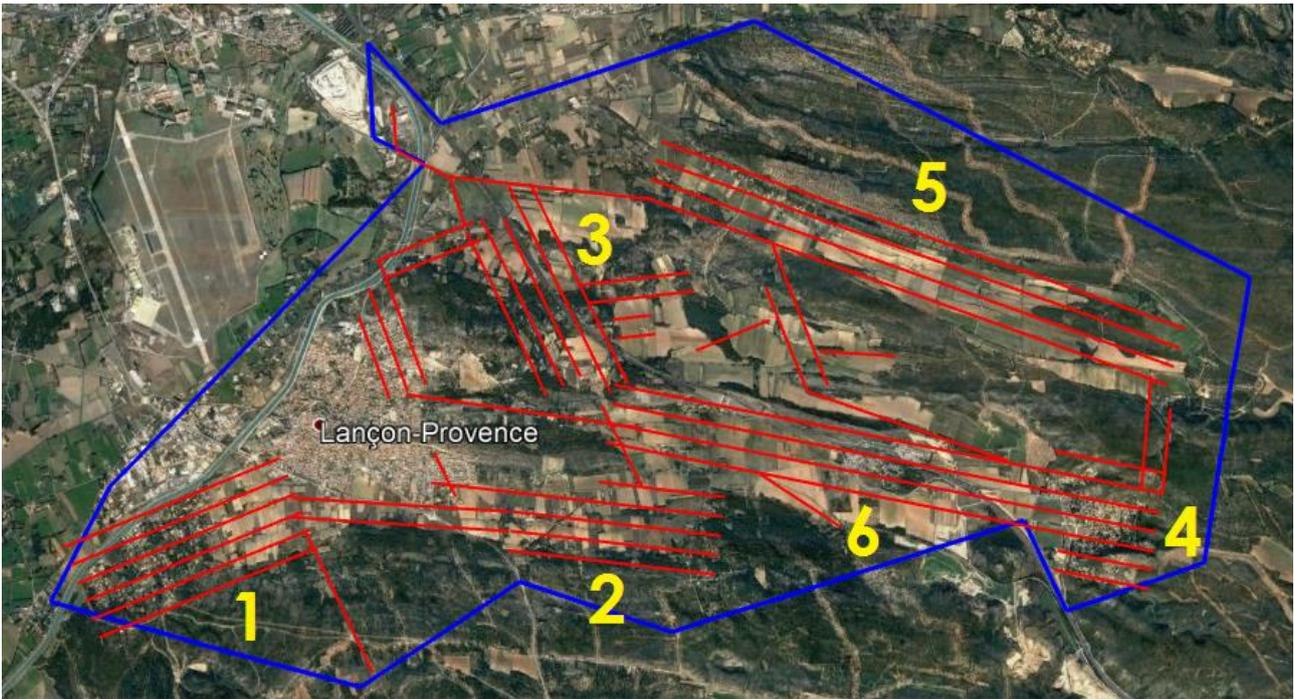
Figure 3.3 Mission plan for the Cabardèle area. The flight paths have been established to cover each sector of the water distribution network.
