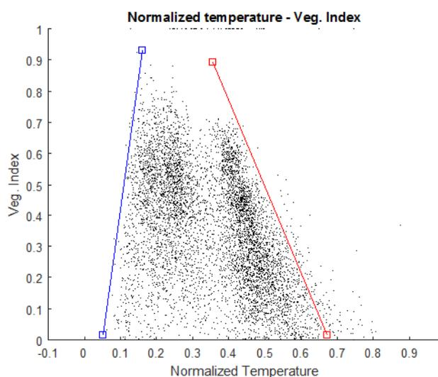
Figure 8.2 Scatterplot between the Normalized Temperature and the NDVI vegetation index corresponding to the waterleaks test field (October 2018).
