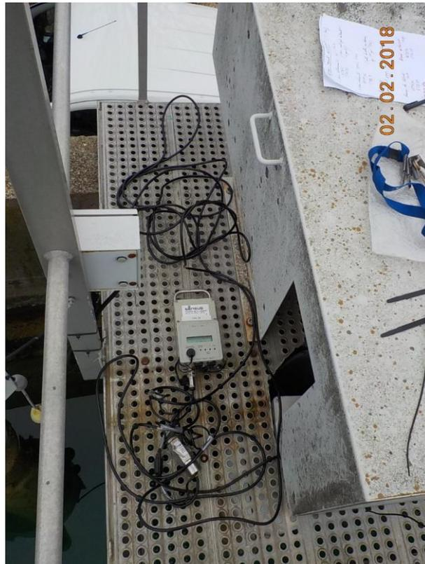
Figure 6.9 Level sensor with data logger.
