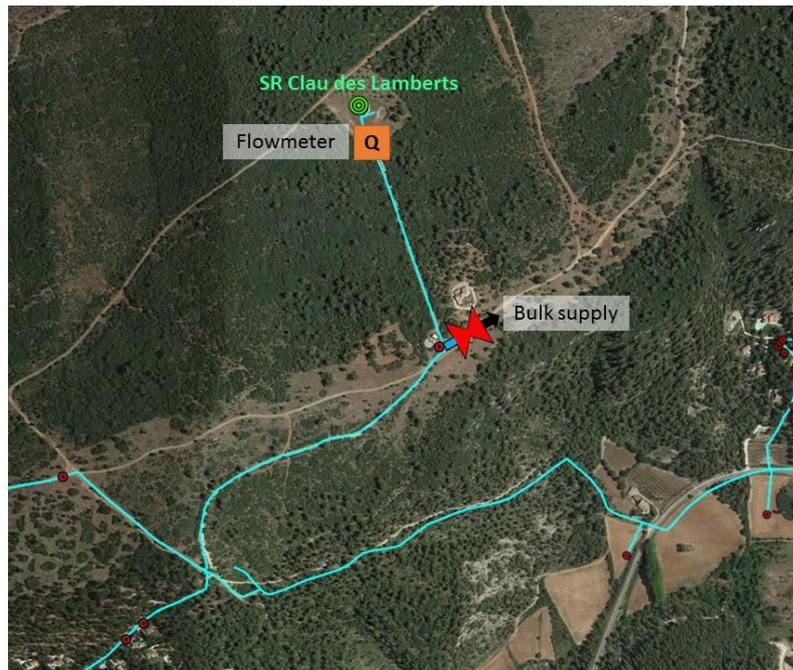
Figure 4.4 Flowmeter installation at Clau des Lamberts SR as per option 2 (bulk supply shall be shut off during the step test).
