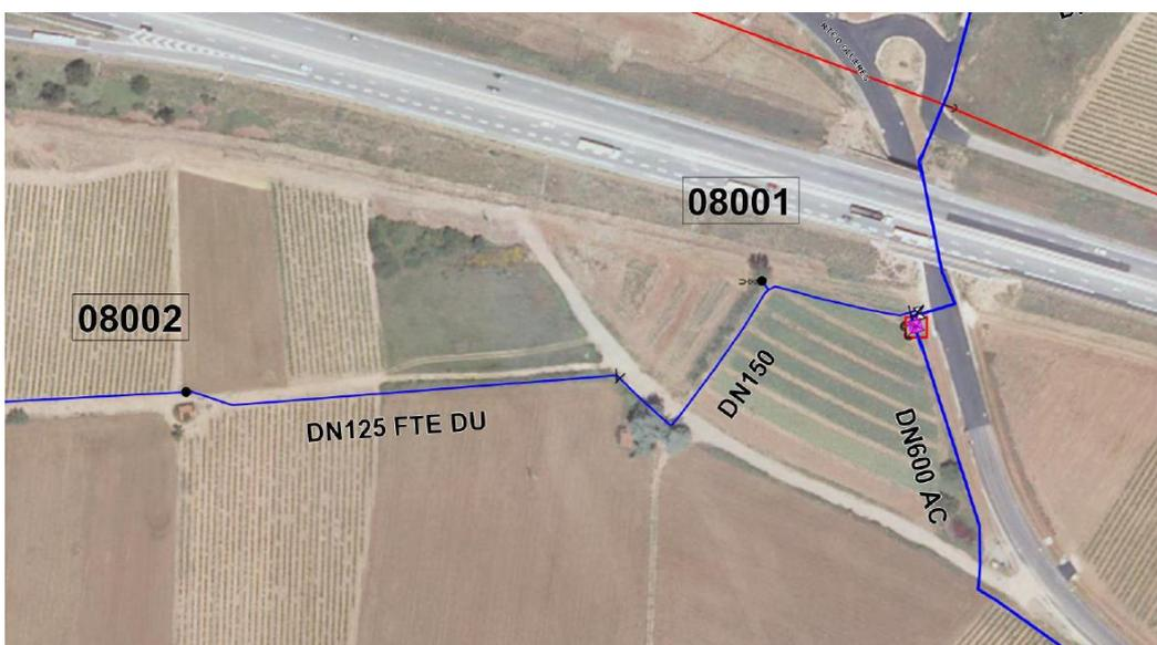
Figure 6.10 Location of flow measurement devices Q2 and Q7.
