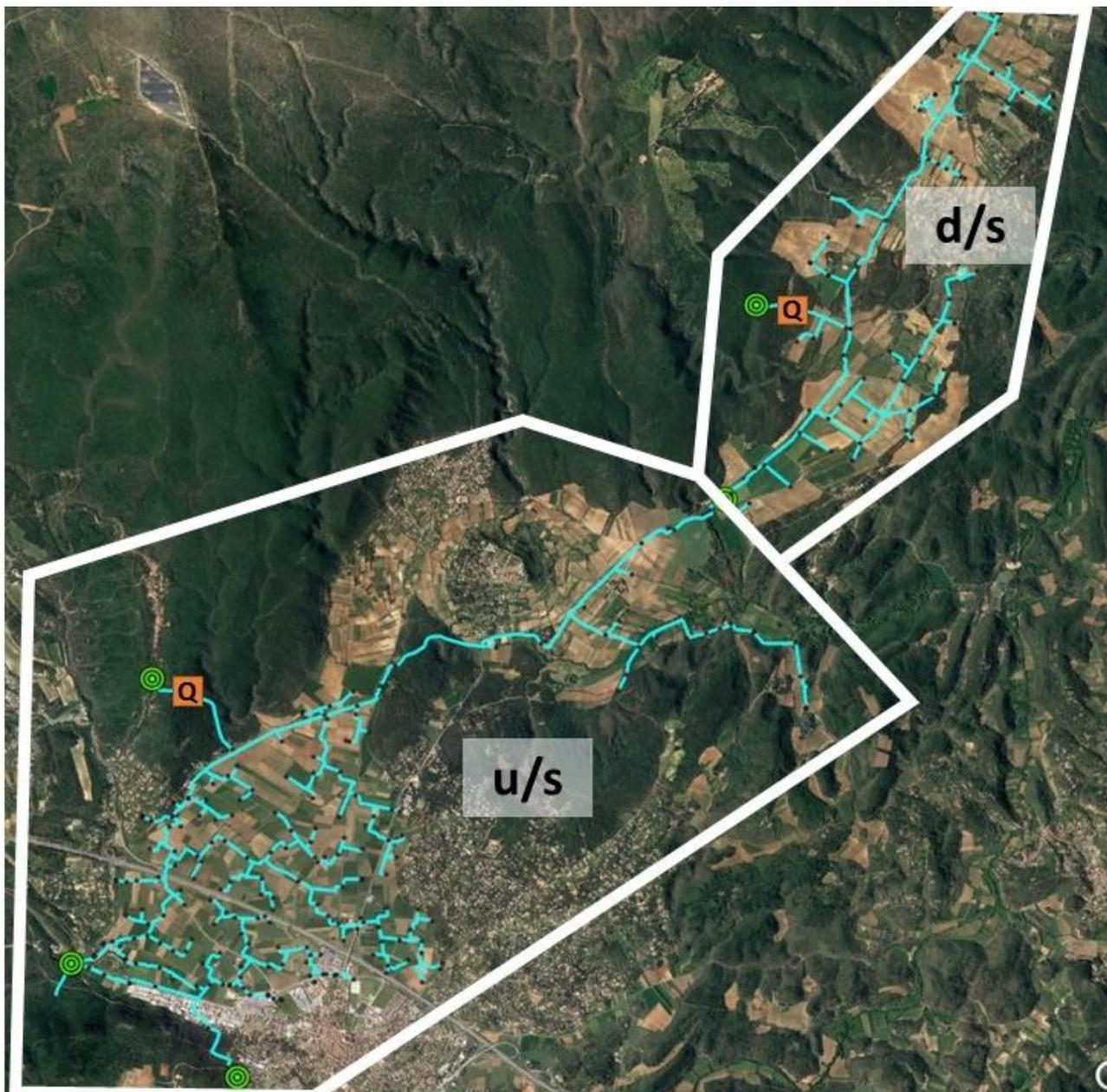
Figure 4.6 Subdivision of Verdagne site into two sub-sites – u/s of BS and d/s of BS – and flowmeters' installation points at Rabinets and Planissard SRs.
