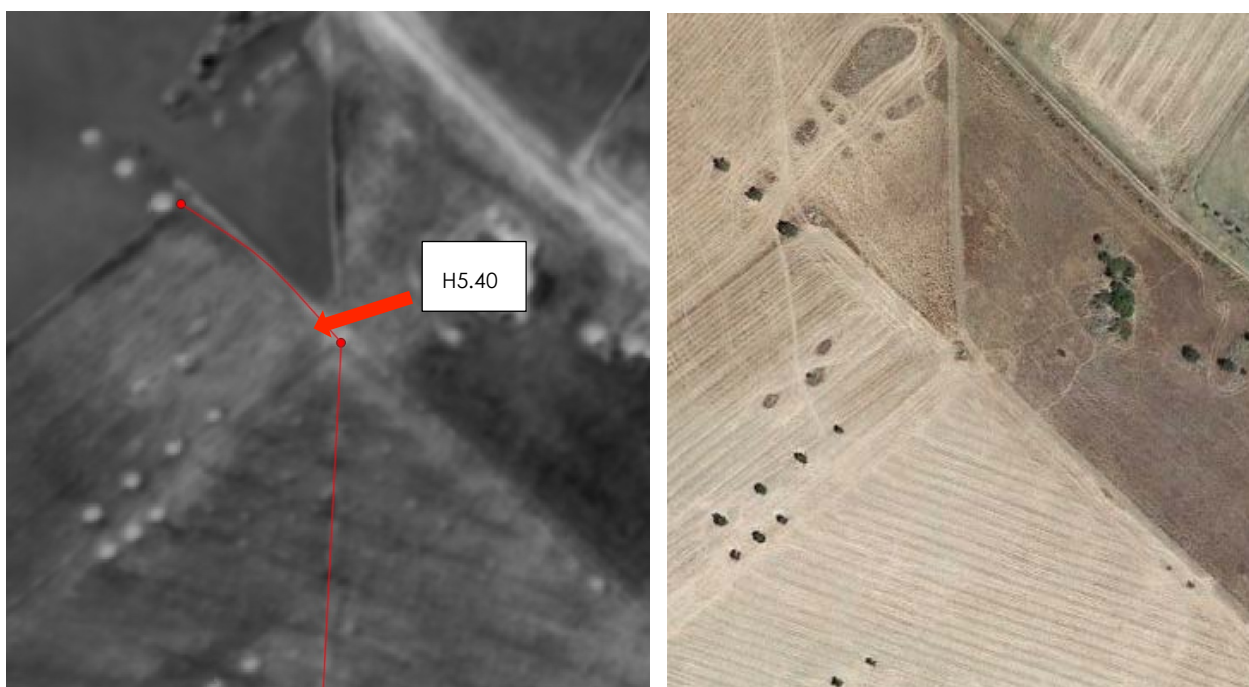
Figure 73 : WI map in the vicinity of hydrant H5.40 (left). The light grey area in the WI image around H5.40 is most probably related to the presence of denser or greener vegetation (as revealed on Google Earth image –right). A small water leak could thus be suspected.
