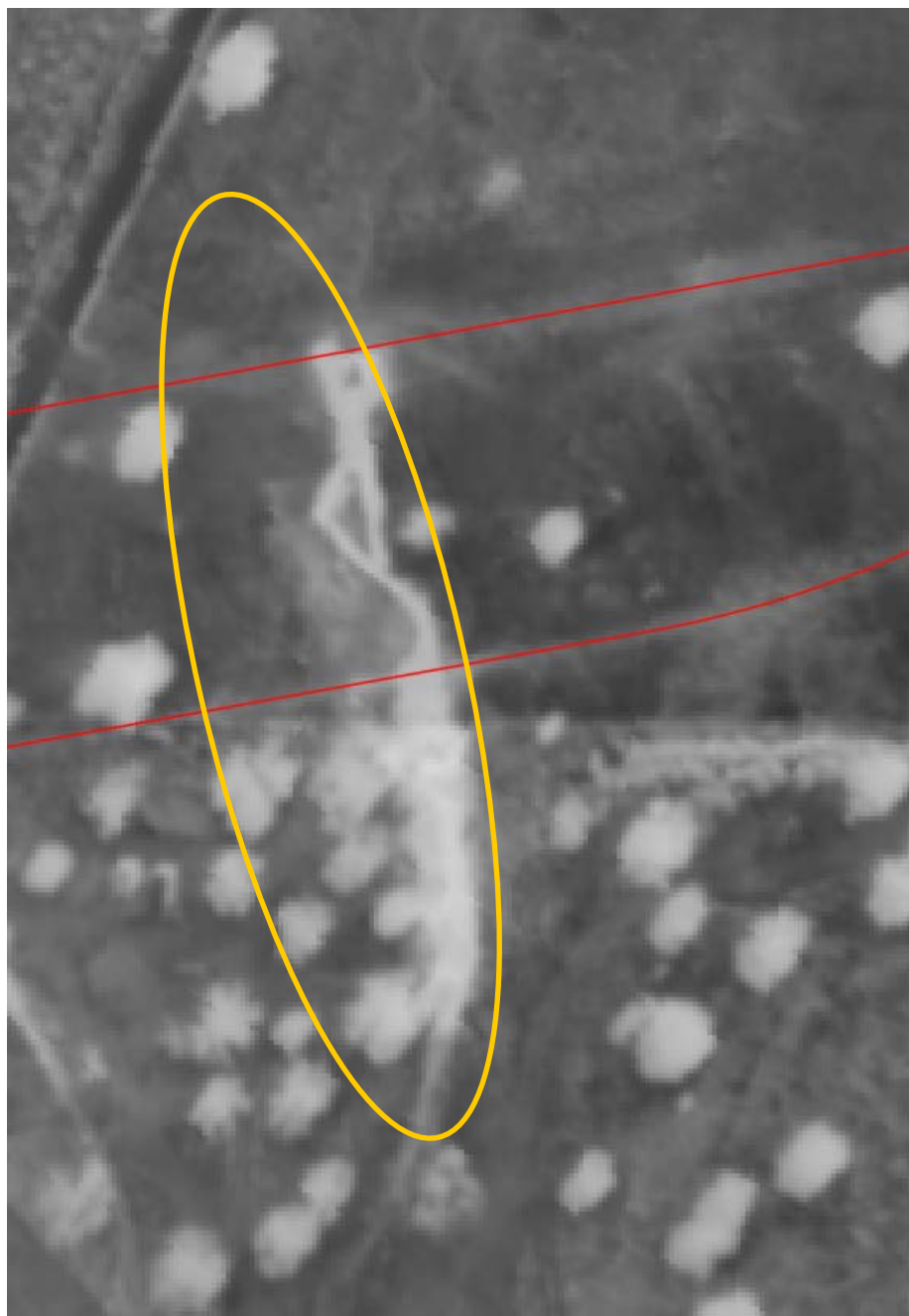
Figure 85 : Vale de Gaio. WI image (Sept. 11th) of a suspected leak west of the reservoir.
