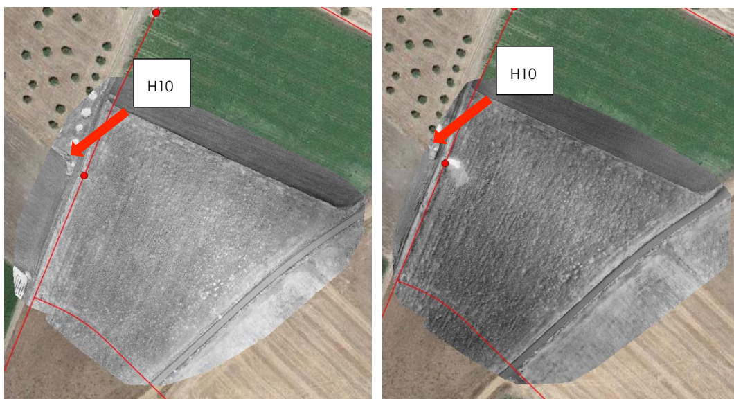
Figure 126 : Artificial leak H10 (left: 14-05-2019: 14:07– and after the vane was opened – right: 16-05-2019: 14:36).
