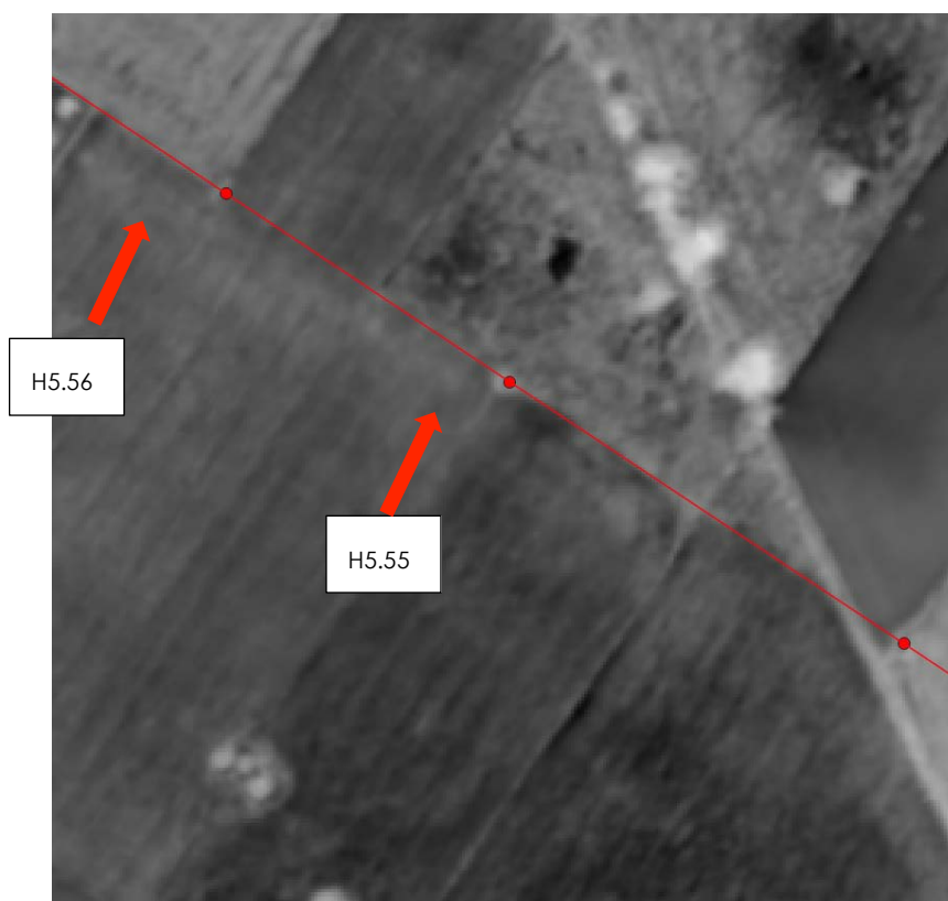
Figure 74 : WI map in the vicinity of hydrant H5.55 and H5.56. Both concrete blocks have the same size, however, the water index reveals a brighter spot around H5.55 as compared to H5.56. It should be checked if there is a difference in soil coverage (green grass as compared to dry grass or bare soil?), which could be interpreted as the presence of a small water leak.
