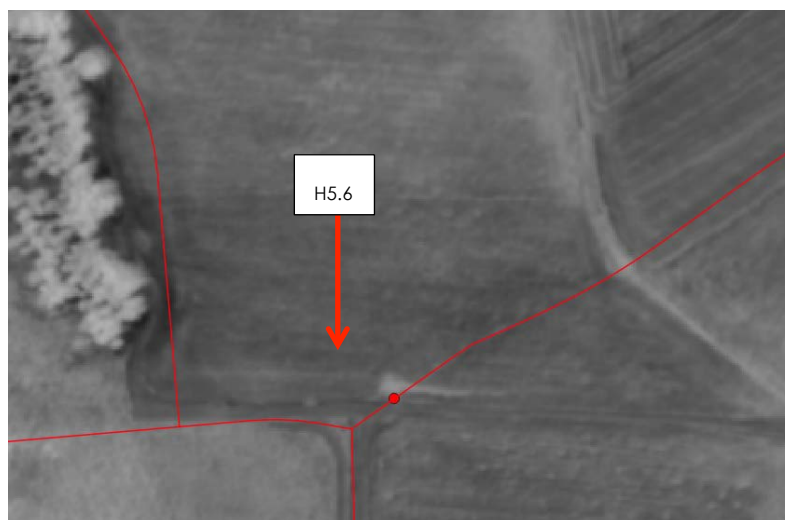
Figure 67 : Moisture map (close up in the area of the artificial leak H5.6) as obtained according to Processing 3, together with the pipeline.
