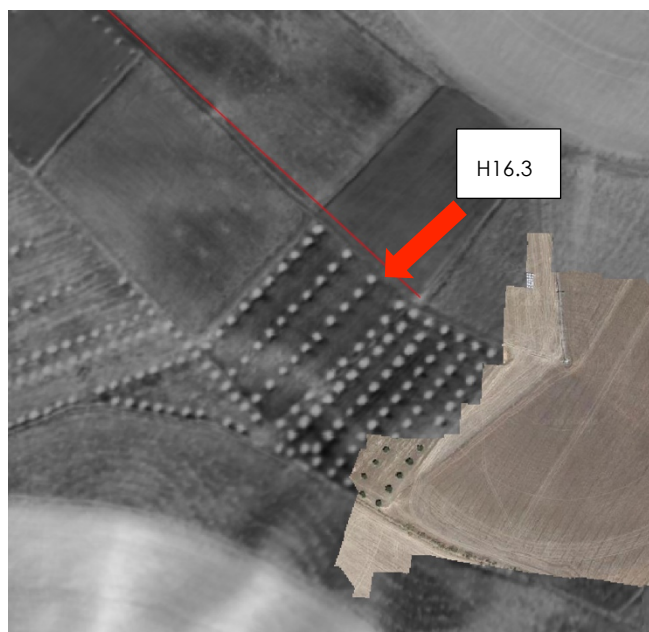
Figure 71 : WI map in the vicinity of hydrant H16.3. A small leak was detected by SGI at this hydrant. A slight moisture contrast (light grey) can indeed be seen in close vicinity of H16.3.
