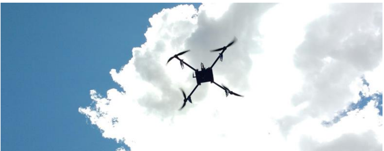
Figure 2.3.3 Multicopter with on-board multispectral and thermal infrared cameras operated by Galileo Geosystems.
