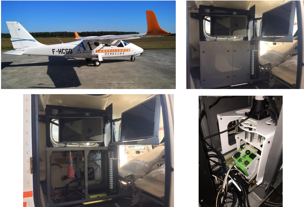
Figure 2.3.2 Gimbal integrated into the AIRMON console of the Air Marine TECNAM
