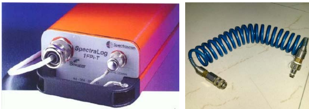
Figure 14 : Data logger able to log both flow and pressure simultaneously (left) and flexible spiral hose to connect the pressure logger to the pipeline (right)
