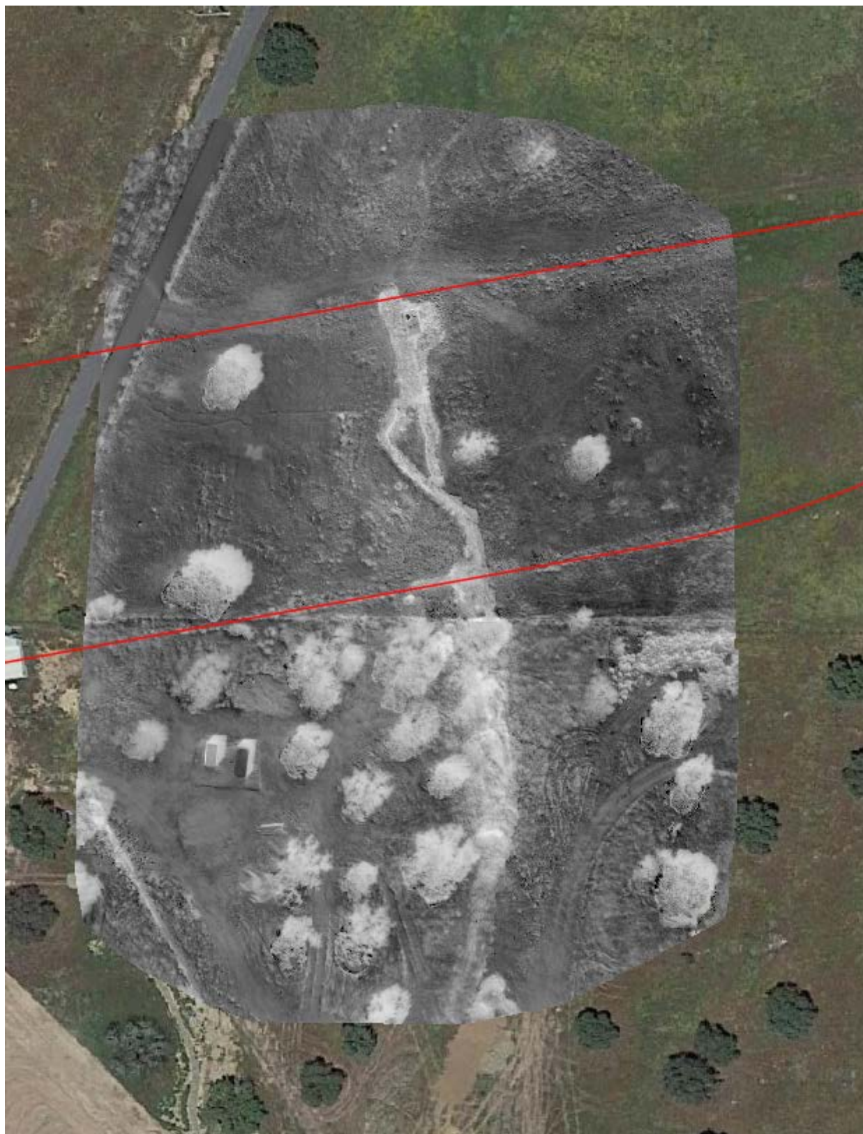
Figure 137 : Vale de Gaio. Water index map of the "leak" west of the reservoir. Sept 11
