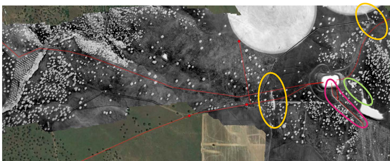
Figure 84 : Sept 11 th . 2019, MAV flight, Close-up of the WI map near the reservoir. Two suspected leaks are highlighted with orange ellipses, Vale de Gaio.
