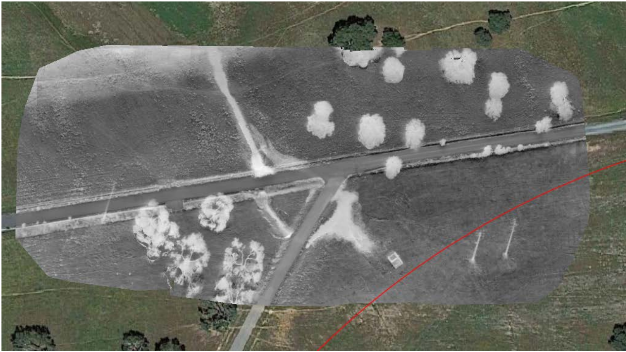
Figure 136 : Vale de Gaio. Water index map of the "leak" north east of the reservoir. Sept 11
