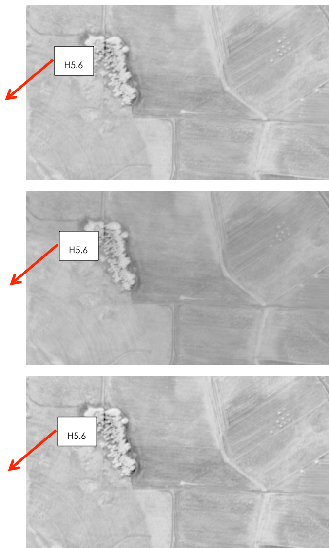
Figure 66 : Moisture maps (close up in the area of the artificial leak H5.6) as obtained according to Processing 1, 2 and 3 (from top to bottom). The leak H5.6 is clearly seen.
